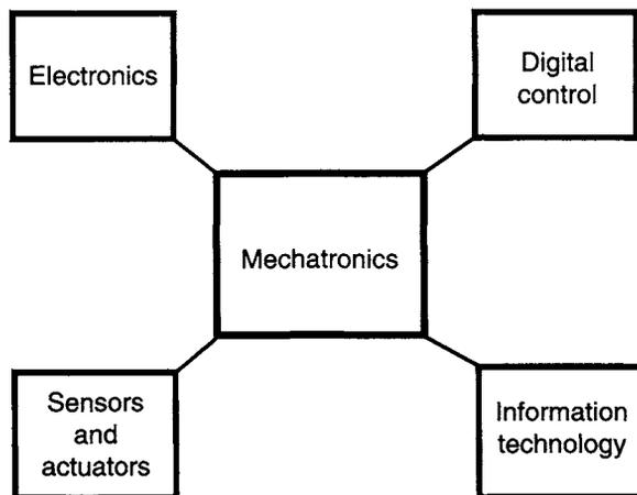
**Figure 1.1** Main components of a mechatronic system.
