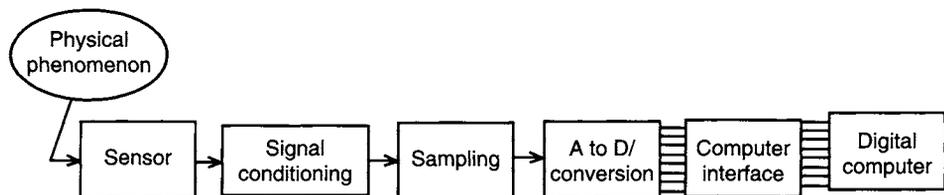
**Figure 1.8** Measurement system.
